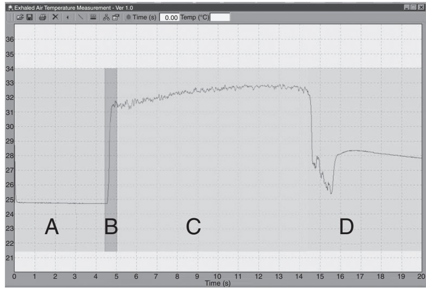
Fig. 1. Temperature/time curve during a slow expiratory manoeuvre from total lung capacity. Part A and part D correspond to the phases of approach and separation from the mouthpiece. Zone B describes the rapid increase in temperature at the beginning of exhalation. Zone C is the segment where the plateau of exhaled air temperature is located.
