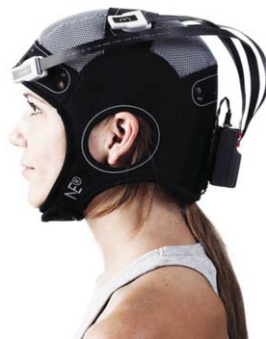
Figure 1. The wireless EEG system “Enobio”
