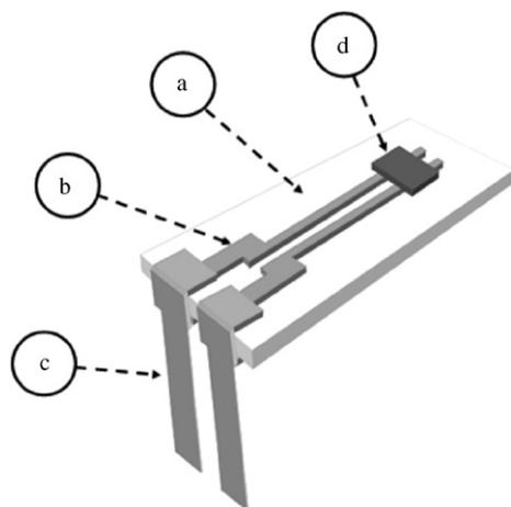
Fig. 1. Sensor layout: (a) alumina substrate; (b) gold contacts; (c) pins; (d) sensing layer.
